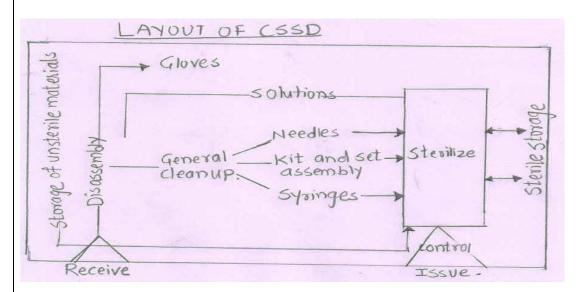
It consists of series of working station in dirty,non sterile area which are separated from sterile by Autoclaving and different sterilizing equipment. In layout, sterile area is established having
